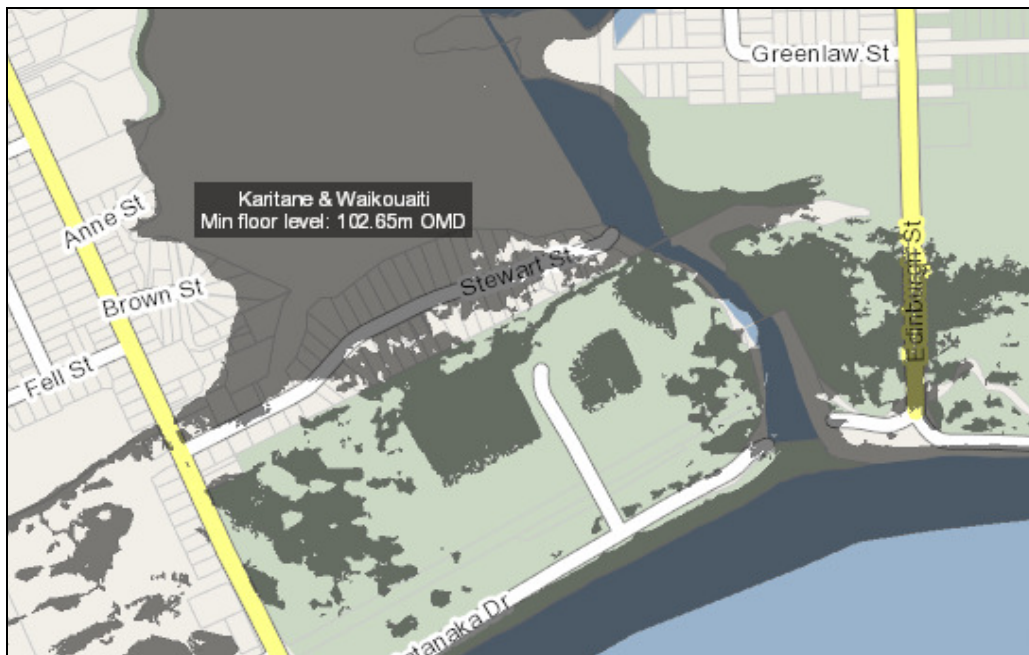
Figure 2.4: Areas at the south end of the Hawksbury Lagoon affected by new local body minimum floor level policy
